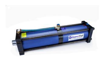
HZ SERIES. The HZ power-stroke-only series is a totally self-contained and cost-effective power source designed for marking, coining, clamping, piercing, riveting, notching, and assembly applications in which short-stroke, high-speed, and high-force operation is required. HZ cylinders provide power stroke only (no approach stroke) and are controlled by a single 4-way pneumatic control valve.
