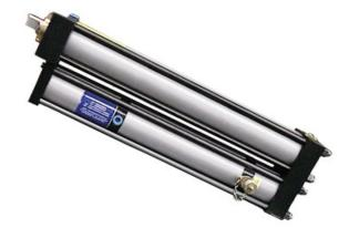
• **NEW HPX SERIES.** The new HPX EXTRA SHORT cylinder series is essentially a satellite cylinder that provides longer strokes with a shorter work cylinder. This is accomplished through its unique design, which pairs a larger booster unit with a smaller work cylinder.
