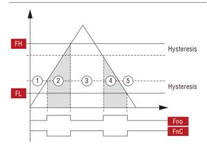
This mode is used to judge whether or not a measurement value is inside or outside of a specified zone.
