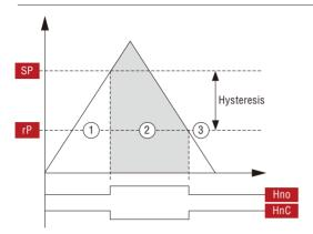
Pressure is likely to fluctuate from factors such as pressure spikes. This mode allows for free adjustment of hysteresis in order to prevent chattering due to fluctuating pressure.
