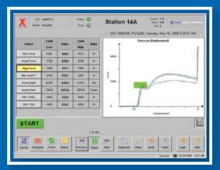
The HyperView-Press® uses Sciemetric's advanced signature analysis technology to eliminate false accepts and find more defects than other press monitoring systems.
