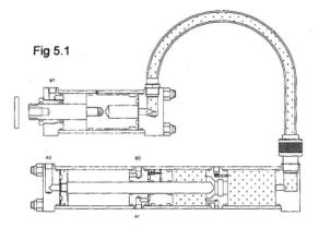
2. Approach Stroke - Air is directed to Port A1. The Reservoir piston advances, displacing the reservoir oil through the valve block to the back of the working piston, advancing the cylinder rod (at low force) until meeting resistance (work surface or part contact).
