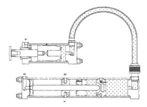
3. Power Stroke - Regulated air pressure is applied to Port A2. The high pressure piston and rod advance contacting the valve block seal and isolating the reservoir oil from the working section. Continued movement of the high pressure rod and piston assembly intensifies and displaces the trapped oil developing the power stroke. Step 1 returns all three pistons and oil to the retracted position.
