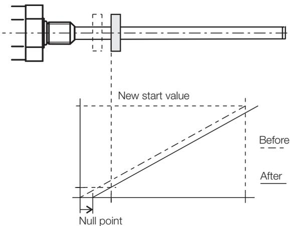
Fig. 6-4: Adjusting new start position (offset shift)
