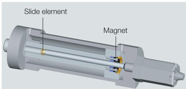
Fig. 4-5: Example 1, transducer installed with sliding element
