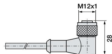
Fig. 12-5: Connector type BKS-S116-PU-\_\_
