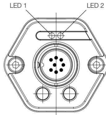
Fig. 3-2: Position of the BTL7 LED displays
