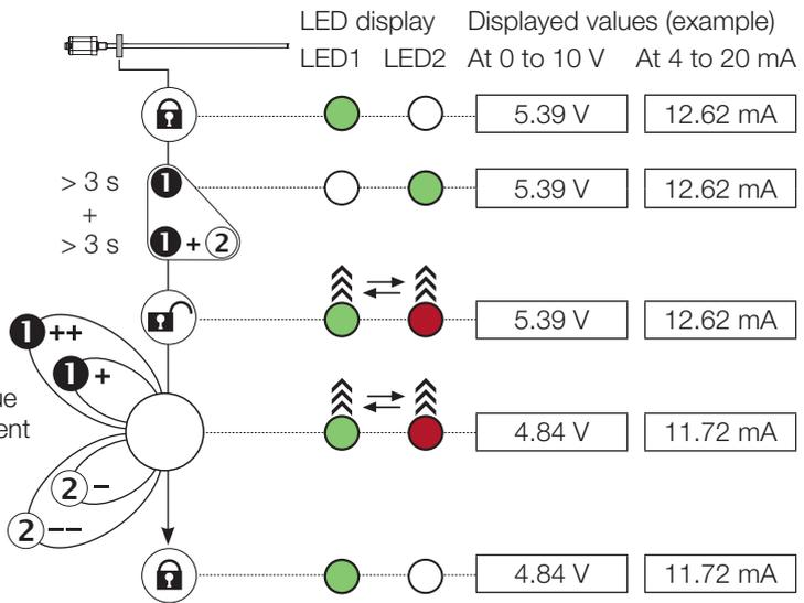
**i** After each calibration procedure you must wait for the lockout time of **15 s**. This also applies to switching between the start value and end value setting.
