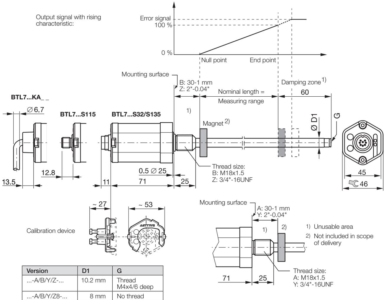
Fig. 3-1: BTL7...A/B/Y/Z(8)... transducer, construction and function
