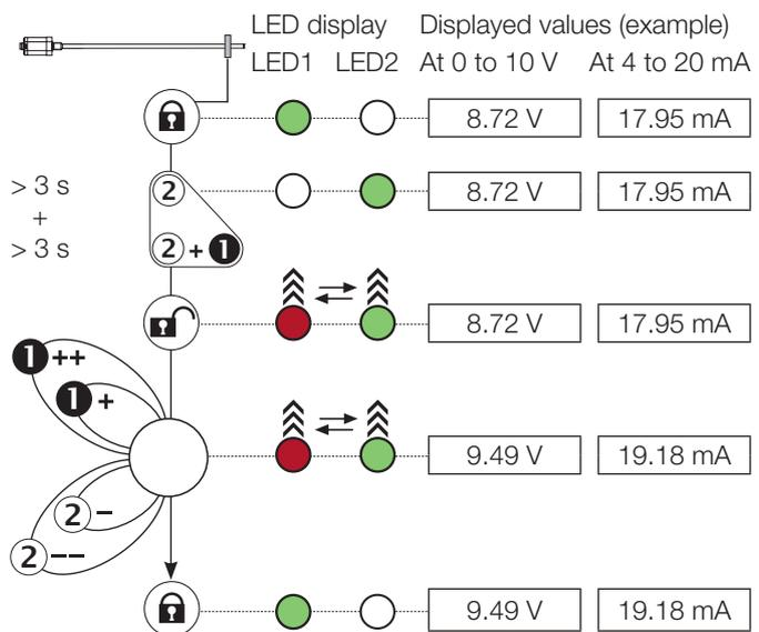
1) Briefly press button: Current value is increased or decreased by approx. 1 mV or 1  $\mu$ A. If a button is held down longer than 1 s, the step interval is increased.
