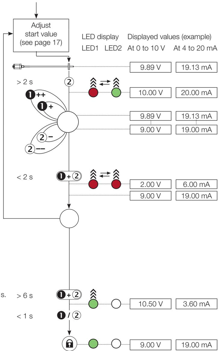
1) Briefly press button: Current value is increased or decreased by approx. 1 mV or 1 µA. If a button is held down longer than 1 s, the step interval is increased.
