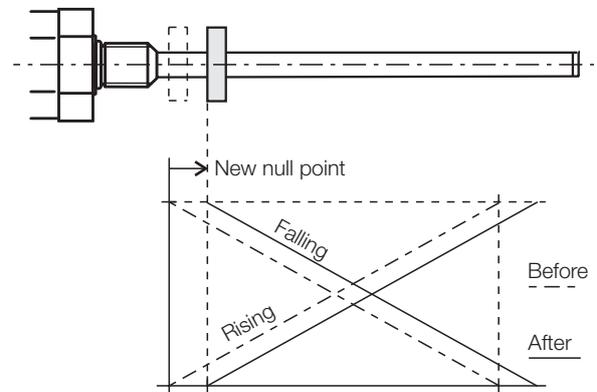
Fig. 6-2: Reading new null point (offset shift)
