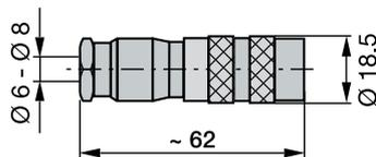
Fig. 12-6: Connector type BKS-S135M-00
