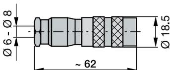
Fig. 12-2: Connector type BKS-S32M-00
