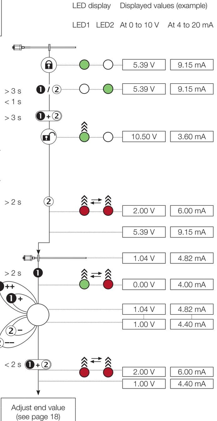
1) Briefly press button: Current value is increased or decreased by approx. 1 mV or 1 µA. If a button is held down longer than 1 s, the step interval is increased.
