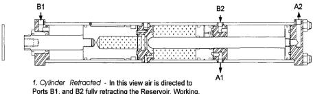
Ports B1, and B2 fully retracting the Reservoir, Working, and High Pressure Pistons.
