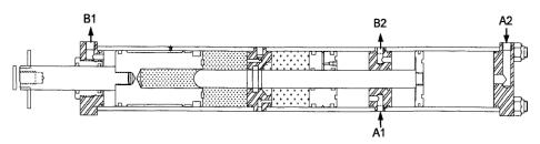
3. Power Stroke - Regulated air pressure is applied to Port A2. High Pressure Piston and Rod advance until contacting the Valve Block seal, isolating the reservoir oil from the oil contained in the working section. Continued movement intensifies and displaces the trapped oil developing the Power Stroke. Step 1 returns all three pistons and oil to the retracted position.
